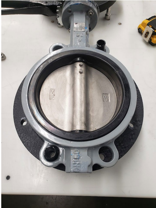
Fig. 1; Butterfly valve with inlet flange & bolts removed.
