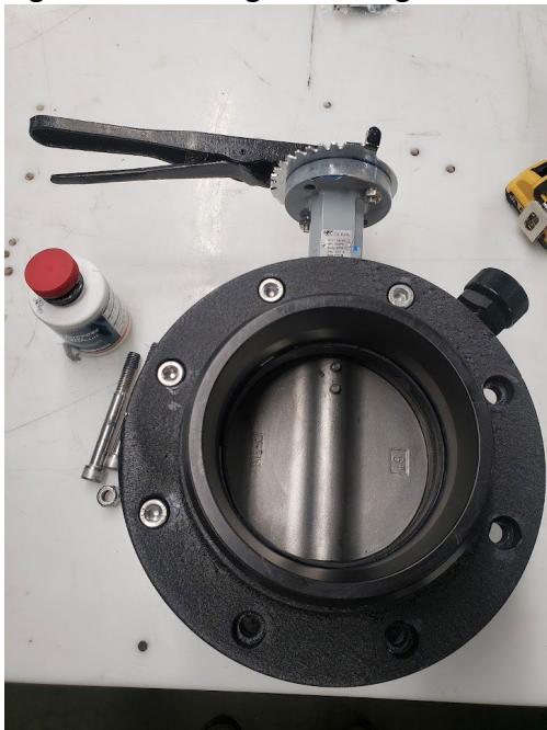
Fig. 2: Reinstalling inlet flange in new orientation.
